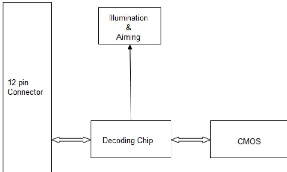
The 12-pin FFC connector on the engine can be connected to a host device with an FFC cable. For information about this cable, please see the "12-pin FFC Cable" section in Chapter 4.
